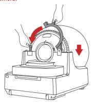
• Remove the refill ring cover, put the refill ring in, and put the cover back.
