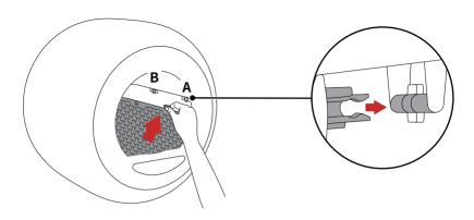
**⑤** Put the cylinder on the base, lock the buckle, and make sure the buckle is fastened.
