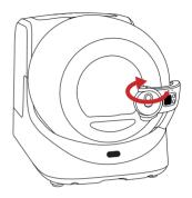
Select the litter sifter according to the cat litter. If it is mineral cat litter, please use the litter sifter P99032. Pour in the cat litter and do not exceed the MAX line. (See 7.1.2 and 7.2.4 for the replacement method of litter sifter)
