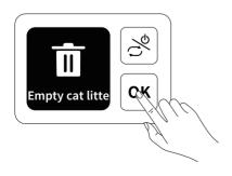
② If the waste bin is full during the emptying process, the device will stop emptying and start auto-packing. After packing, please take out the packed trash bag, and then double press ok to start auto-refilling.
