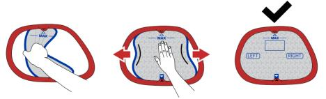
If the blue edge is not visible, the installation is successful.
